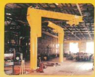
MBAT ICON cranes are designed and manufactured in ordance with IS-807 / 1963 and IS - 3177 / 1977 (revised). MBAT cranes are ideal for wide ranging applications in dustries and are most reliable, robust and yet economical.
